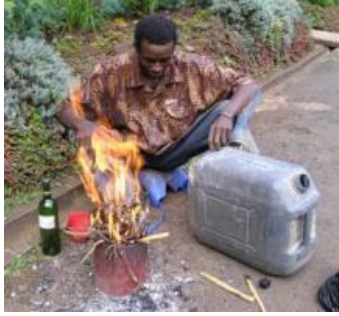
Repairing a jerry-can
